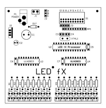
Along with sixteen LED displays, sixteen individual connections are provided just below each LED where you have the ability to connect custom accessories such as lamps, motors or solenoids. These will be toggled on and off at the same time as the LEDs are controlled.
