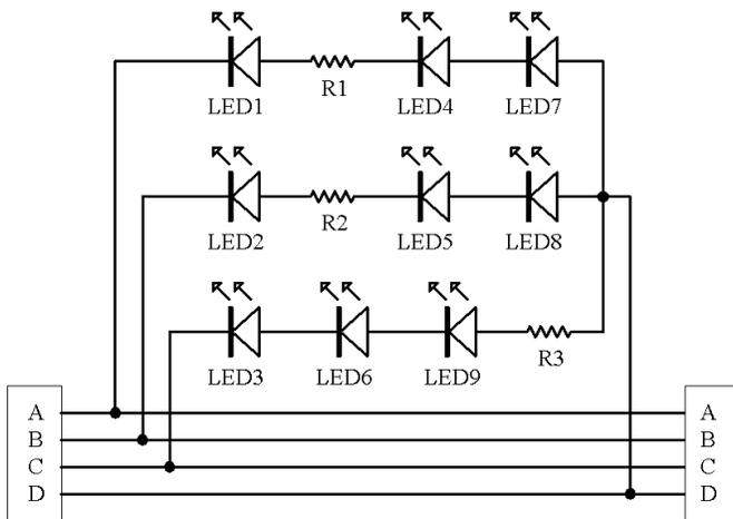
The **LED TriLight** board design allows for power input to be applied to the left or right sides of the board. Total power consumption of a properly configured **LED TriLight** system should be about 60mA in total. Another design feature of our board allows for the power to be drawn off the opposite side of the board to run a second board. The daisy-chaining process has been proven to handle 10 boards connected end-to-end without problem.
