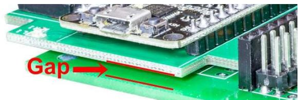
When installing the NodeMCU carrier module, leave a small gap of 1/16"-1/8" (2-3mm) between the bottom of the processor carrier and the **NodeMCU IoT Experimenter**. This ensures traces from the processor board do not short against traces on the main board.
