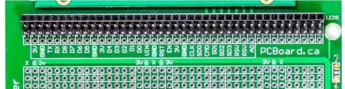
The prototype area on the board has over 1,000 plated 0.1" spaced holes. All processor pins extend to a set of four rows just below the **NodeMCU** and are labeled with their corresponding functions.
